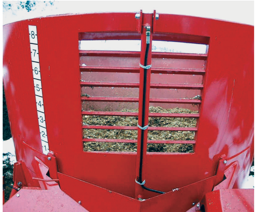
Figure 1: The mixing operation can be observed from the driver's seat through the inspection window up to a certain degree of filling.
