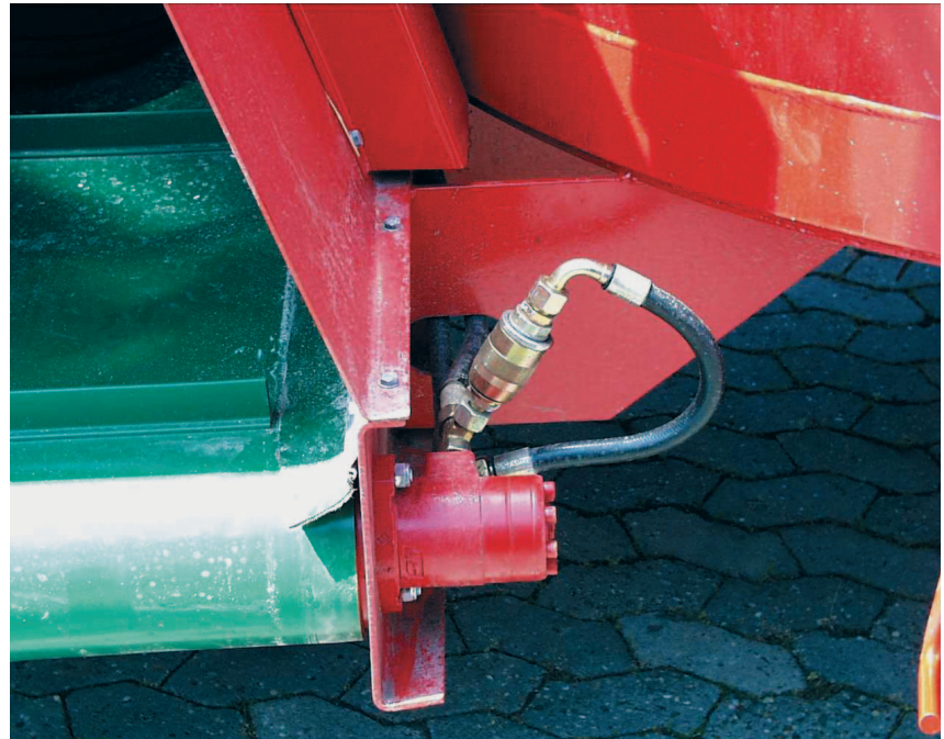
Figure 5: The discharge speed of the conveyor belt can be adjusted individually by the choke valve.
