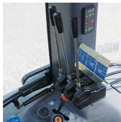
Figure 6: The levers of the Bowden cable control are easy to reach from the driver's seat and comfortable to operate. However, this requires that they are firmly and stably installed at an appropriate place.
