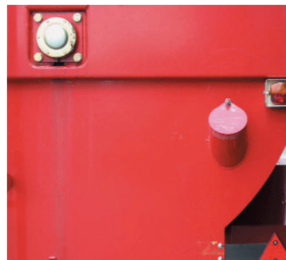
Figure 5: The filler neck at the rear of the mixing container allows small or liquid components to be added.
