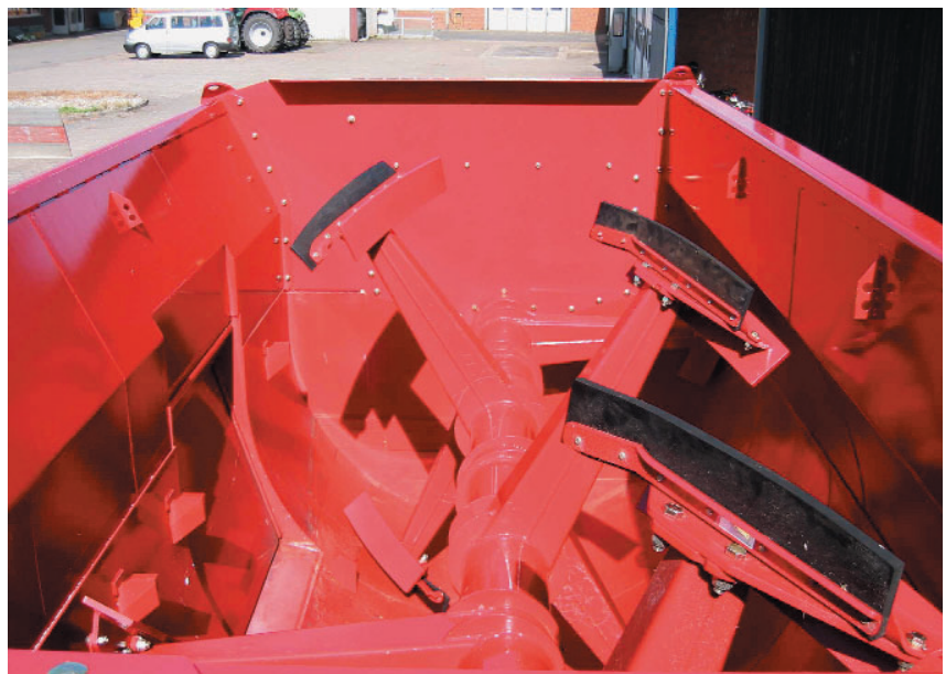
Figure 1: The nine paddles mix the feed extraordinarily gently. The duration of the
