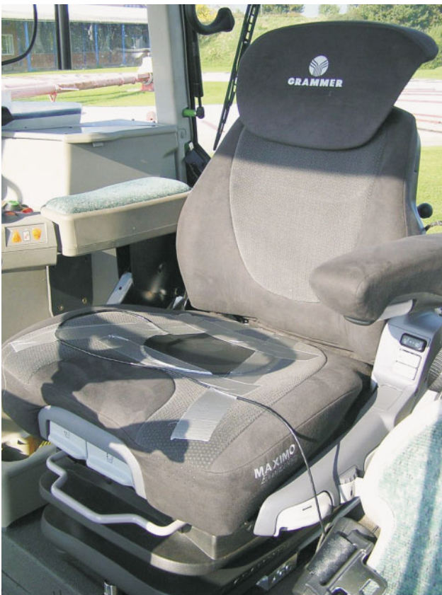
Figure 1: Grammer seat MSG 95 EAC/741 in the tractor with measuring equipment.
