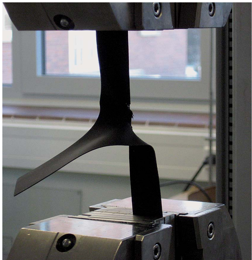
Figure 3: Test of tear resistance at the DLG Test Center
