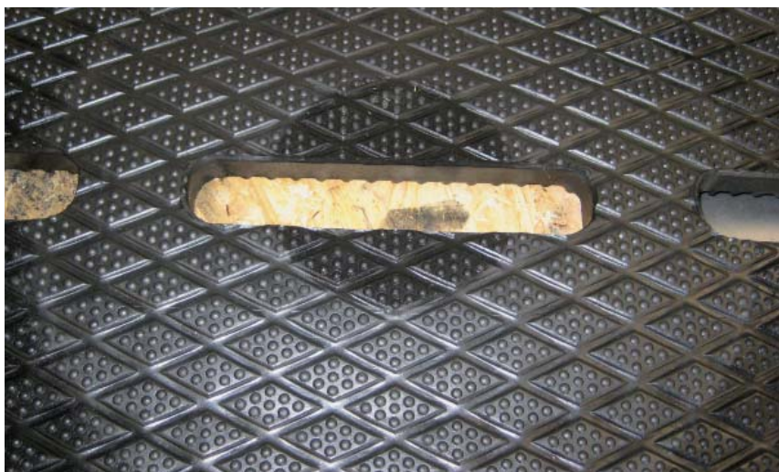
Picture 4: Sample after the permanent tread load
