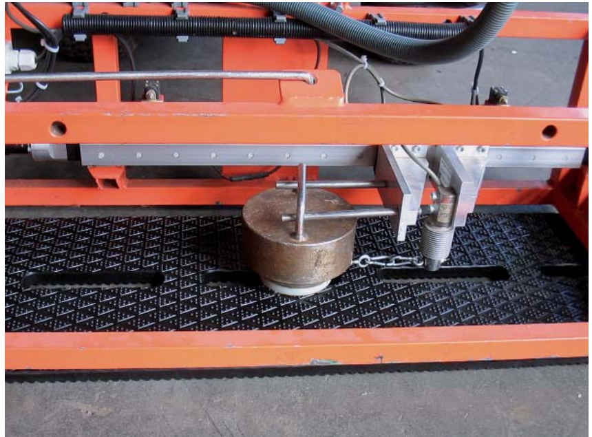
Picture 5: Slip resistance test
