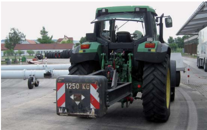
Figure 2: The tractor linkage triangle with ballast carrier and ballast mounted on the test tractor during the endurance/fatigue testing.
