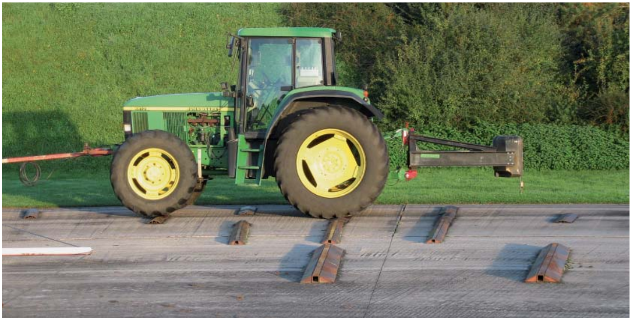
Figure 5: The tractor linkage triangle with ballast carrier and ballast during the endurance/fatigue testing.
