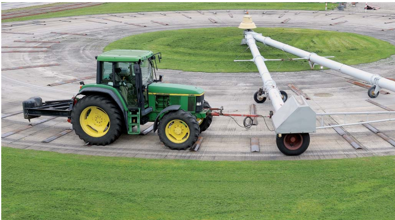
Figure 3: The tractor linkage triangle with ballast carrier and ballast during the endurance/fatigue testing.
