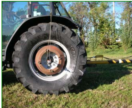
Fig. 9: Tractor equipped with BKT Agrimax RT 657 tyres during traction tests on grassland.
