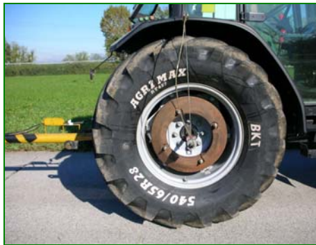
Fig. 10: Tractor equipped with BKT Agrimax RT 657 tyres during traction tests on a concrete track.
